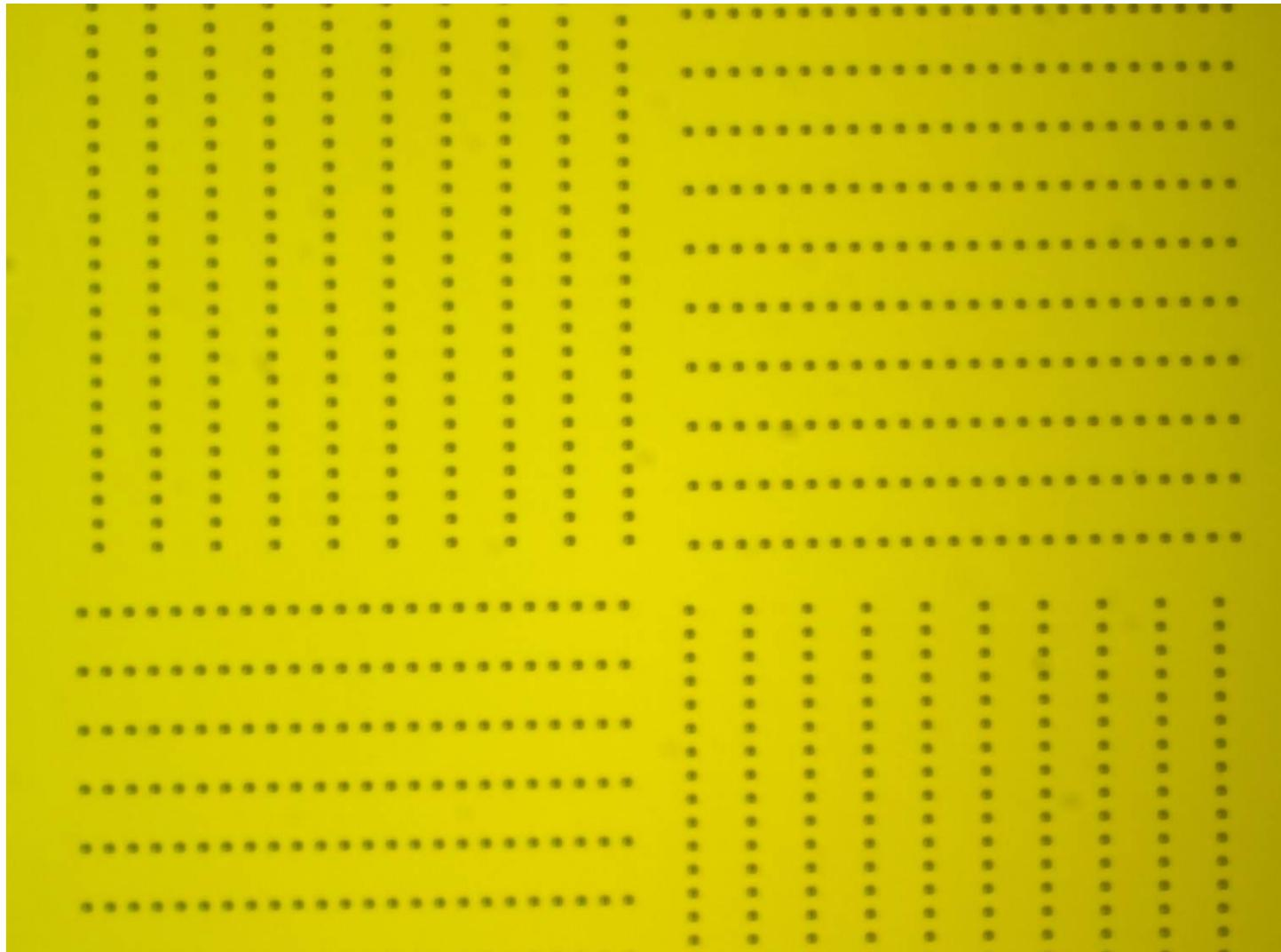
Figure 4. Microscopic pictures after the metal (Ti/Pt/Au: 100/300/2000 Å) lift-off in RR5 resist rempver at 80 C for 5 hours (not lift-off), then, in Acetone (2') and Methanol (1') in ultrasonic bath (only partially lift-off).
