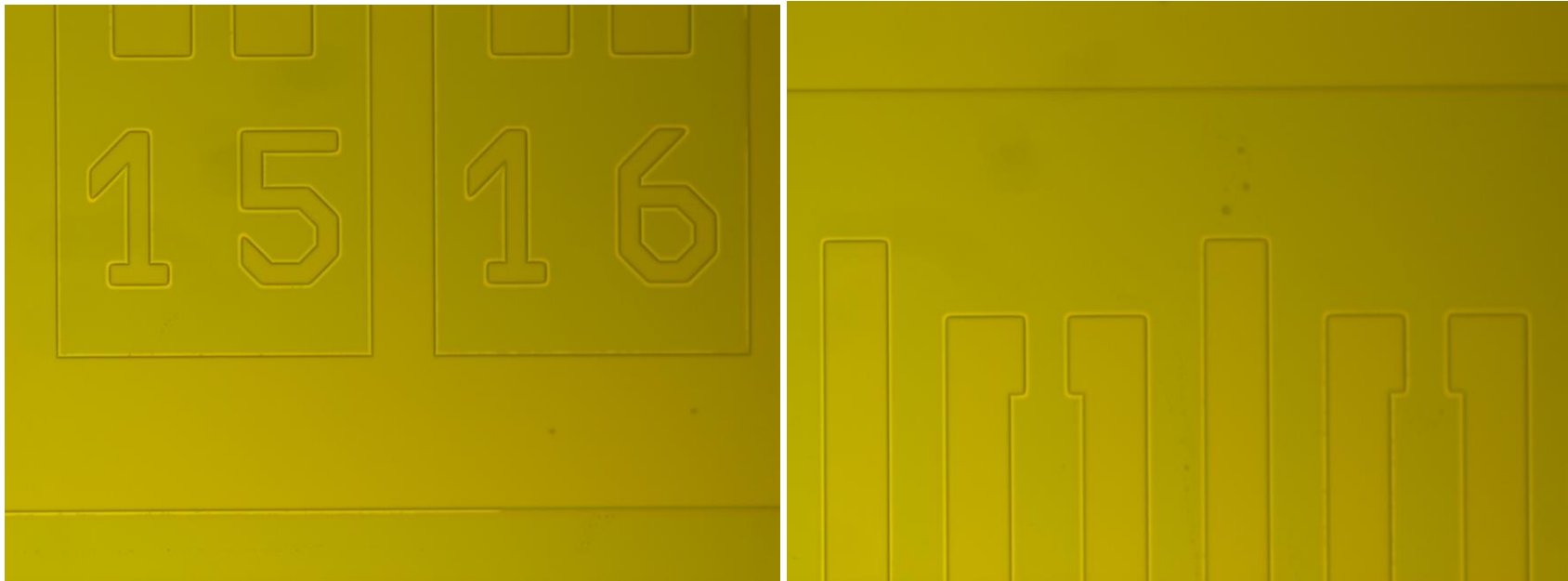
Figure 1 Microscopic pictures show the pattern, with the PR etch mask still on the top and a clear undercut along the resist edge, after 35-minute HCl-solution etch.
