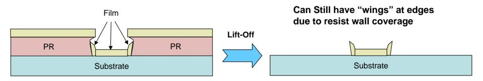
Method #2 (Negative/Image Reversal Resist): By using a negative resist and adjusting the exposure and develop time, one can obtain a retrograde profile. This is much better for lift-off than positive resist which gives a straight or slightly graded profile. Remember, with a negative resist, less exposure means more developer attack which means more undercut.
