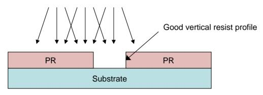
Film Covers All PR edges (No where for solvent to remove PR)
