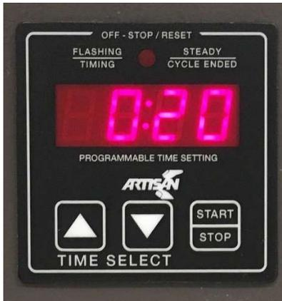
23. Press the START/STOP button to start the timer and turn on the RF power. The green RF ON LED on the RF power supply should illuminate.
