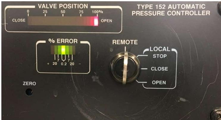
20. Use the CHAMBER PRESSURE CONTROL dial to slowly adjust the chamber pressure (PRESSURE display) to the desired value.
