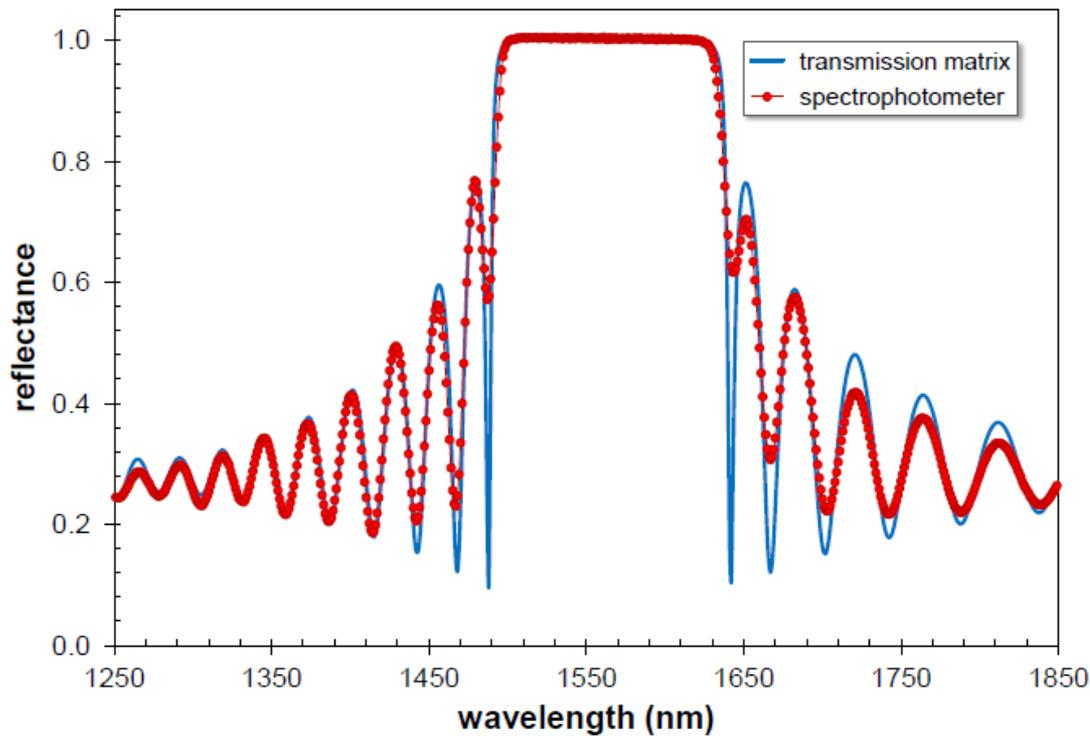
Interference leads to rapid decay of optical field in Bragg reflector
