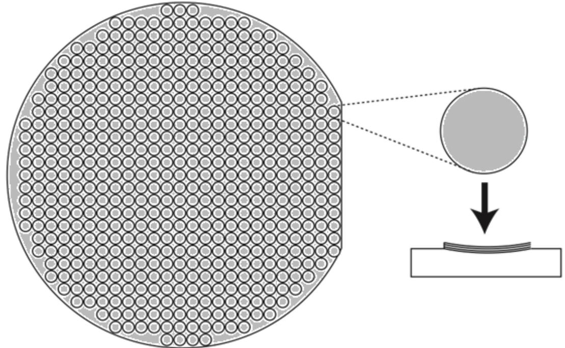
**Wafer-scale batch fabrication enables the generation of many GaAs/AlGaAs mirror disks, though bonding remains a serial process**
