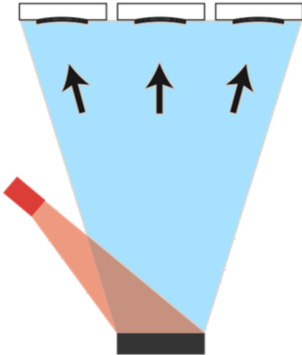
**Physical vapor deposition can be realized on multiple substrates simultaneously**
