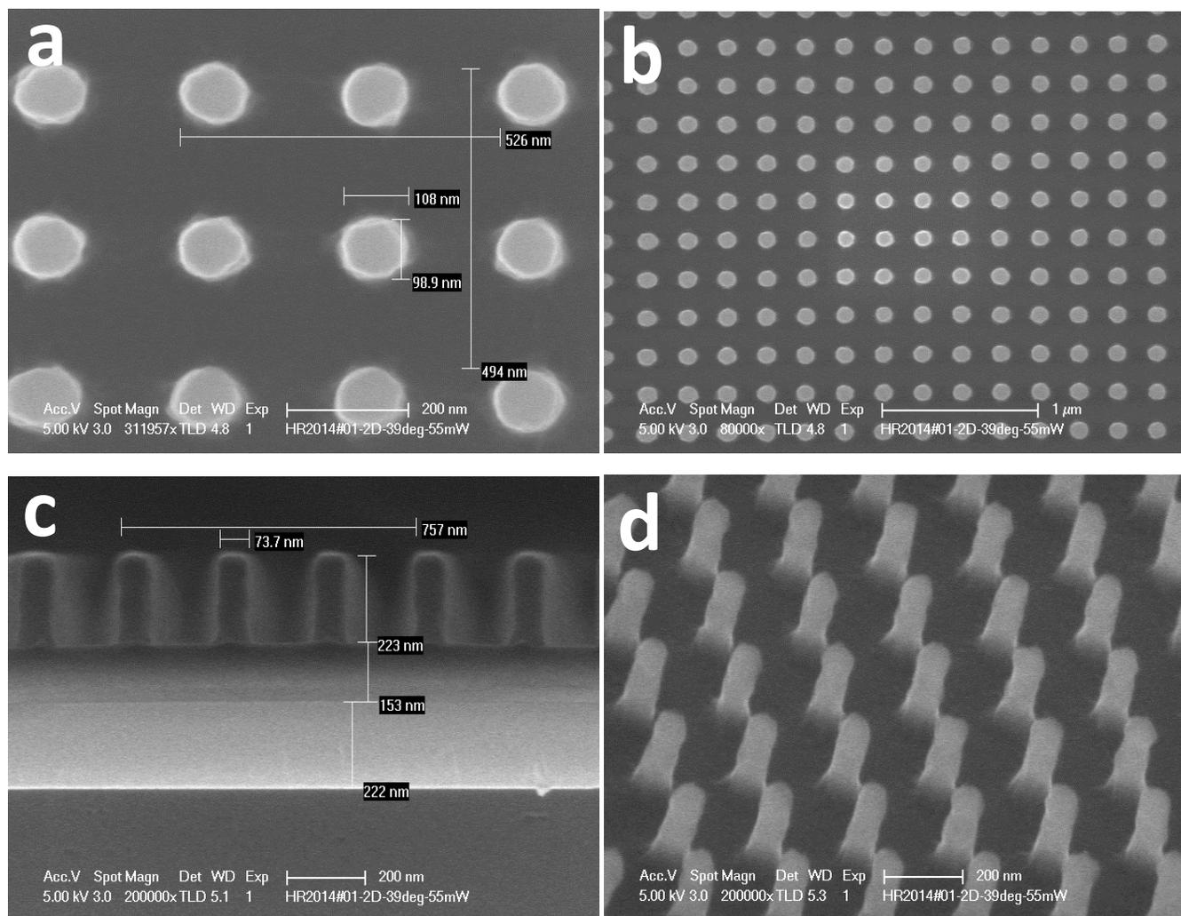
**B) Etching XHRiC-11 (ARC) Layer using RIE#5**
