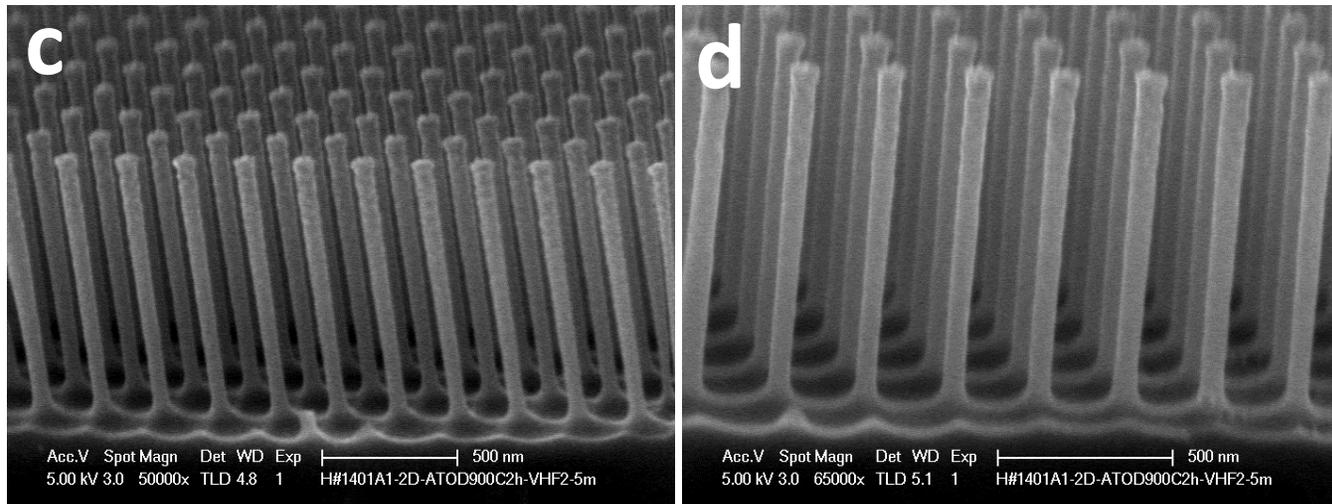
The averaged diameter of the nanowire is 61.0 nm.
