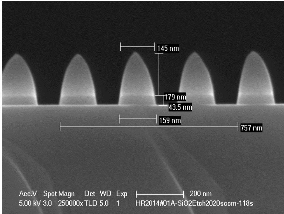
**Note:** The SiO<sub>2</sub> was over-etched into Si as seen in above figure.
