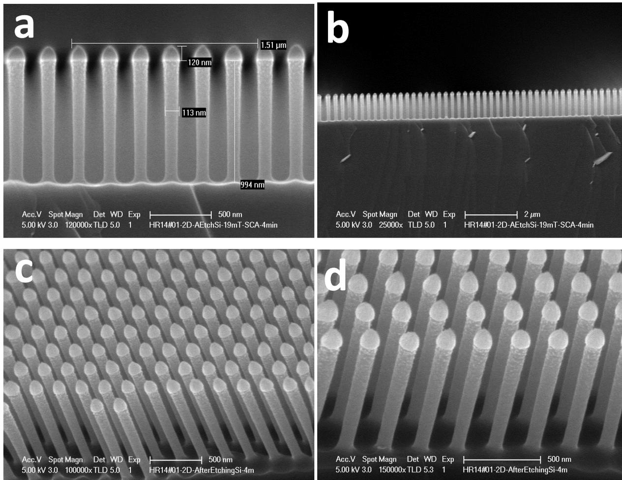
The average diameter of Si nanowire is 106.8 nm
